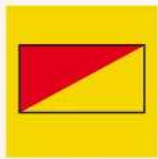
Fire alarm panel
