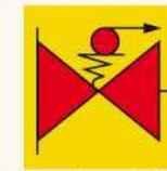
Remote controlled fuel/lubricating oil valves
