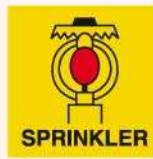
Space protected by sprinkler
