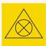
Remote ventilation shutoff
