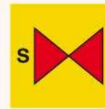
Sprinkler section valve
